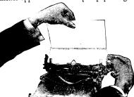
Then bring remainder of sheet forward until it touches portion you have fed through. By a slight prossure on paper release, free paper enough to permit of swinging it to left or right until corners of fed portion coincide with edges of the portion held in hand. (See illustration.)
