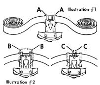
Attach end of new ribbon to empty Spool and wind it around until the eyelet (in all Underwood Corporation Ribbons) reaches inside of Spool. Insert Spools on Ribbon Shafts making sure that the pin at side of Ribbon Shaft is in hole in ribbon spool and that ribbon feeds around front of both spools and through the slots in Automatic Ribbon Reverse Arms.
