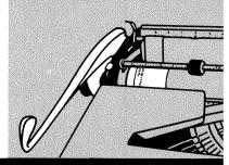
**ERASING** All typists make errors so it is important to know how to make erasures clean and neat. An erasure shield always helps. Move Carriage to right or left so the particles of rubber, grit and paper will fall outside the machine. Place a heavy card directly in back of sheet to make an erasure, or place pieces of paper between each carbon and sheet.
