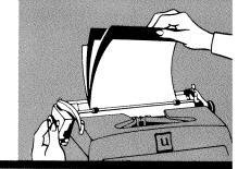
**GAUGING BOTTOM OF SHEET** There are two easy methods: (1) Number vertically a sheet of paper and cut it about a one inch width with enough length to make ends meet around the left end of the Cylinder. Fasten with scotch tape. Insert sheets to align with No. 1. Observe the number where you finish the first page and be guided accordingly thereafter. OR— (2) Insert paper so a slight edge protrudes beyond the edge of the Cylinder and you can easily see your progress toward the bottom of the page.
